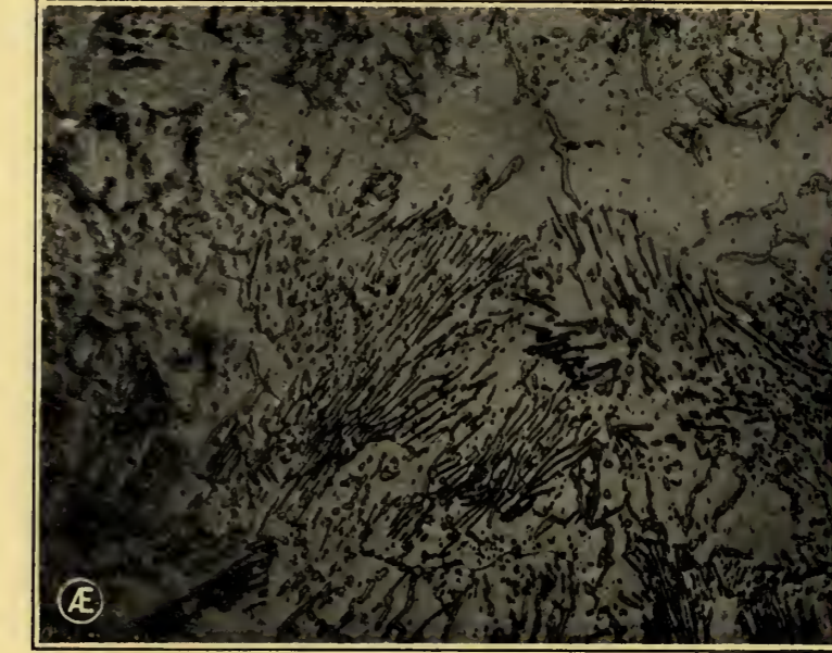
Fig. XIV. Coarsely laminated Pearlite in annealed steel.
