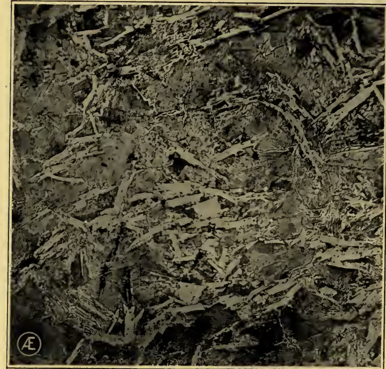
Fig. XVIII. 2.02% carbon steel magnified by 500. Showing more Cementite embedded in Pearlite. †
