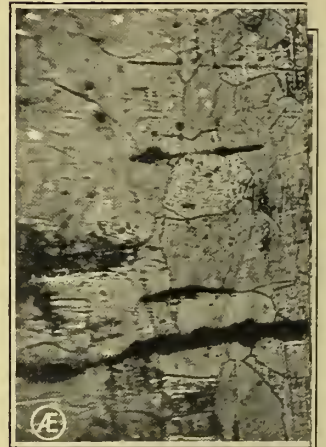
Fig. IX. Ordinary wrought iron with large strips
