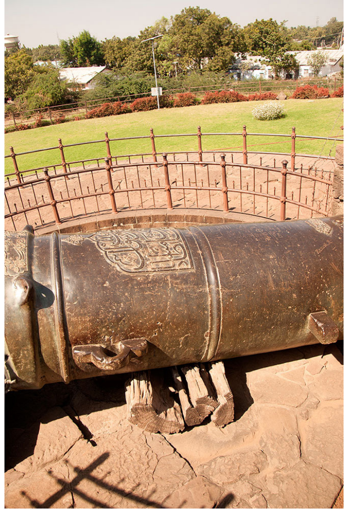
Holding hooks was attached to the cannon for transport or to move the cannon.
